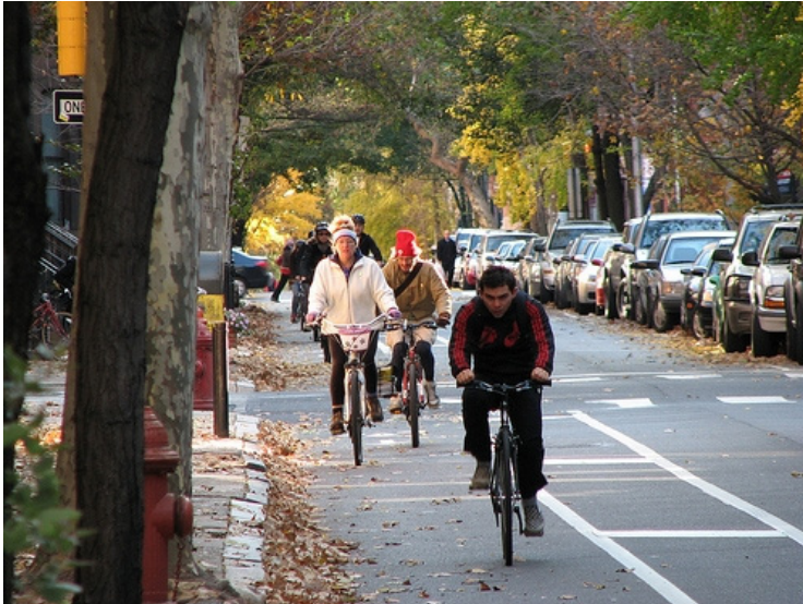
Figure 13: Buffered Bicycle Lane
