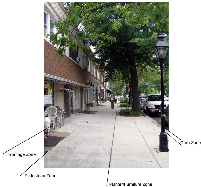
Figure 1: Sidewalk Zonal System
